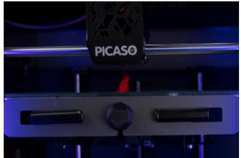
12. Pull the filament feed tube through the guide hole and insert it into the PH against the stop. Make sure that the tube is completely inside the printer and press the joystick.
