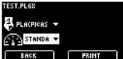
The nozzle and the platform are heated up to the operating temperature. The printer starts an automatic calibration of the workspace coordinates and starts printing a model, such printing takes no more than an hour. The current status and estimated print timing will be displayed on the screen.
