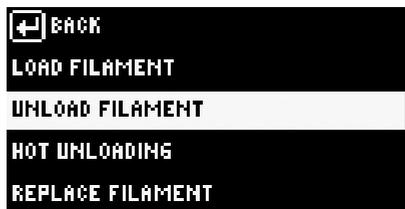
2. The printer starts the algorithm for unloading the material out of the PH along with heating up to the unload temperature in compliance with settings of the selected profile.
