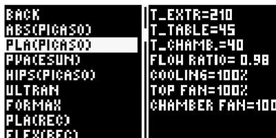
4. The printer starts the algorithm for heating the nozzle up to the operating temperature in compliance with settings of the selected profile. After reaching the operating temperature, the printhead moves to the filament load position. A ready message is displayed.
