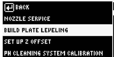
2. The printer starts an algorithm for heating up the platform and nozzle to the operating temperature in compliance with settings of the selected profile. Heating is necessary to eliminate the effect of filament residues on the build plate leveling result. When the operating temperature is reached, the printhead (PH) moves to start setting position.
